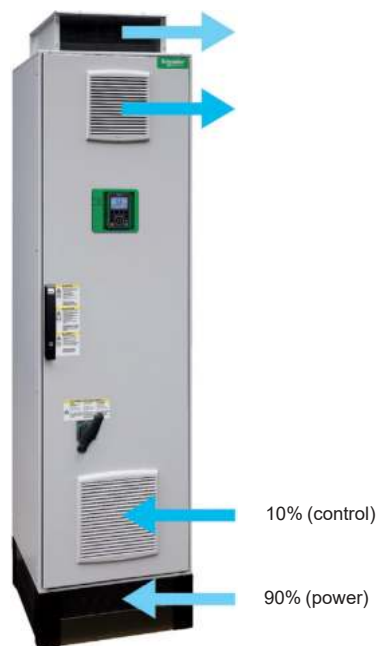
Cooling system with two separate air flows
